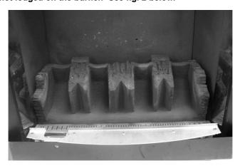
b) Place the left hand front coal rail moulding onto the front ceramic rail support as shown below in Fig. 3
