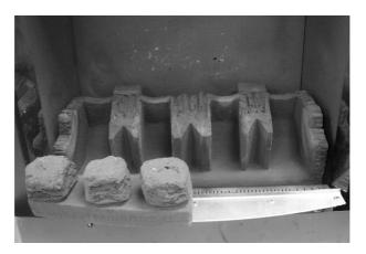
c) Place the right hand front coal rail moulding onto the front ceramic rail support as shown below in Fig. 4
