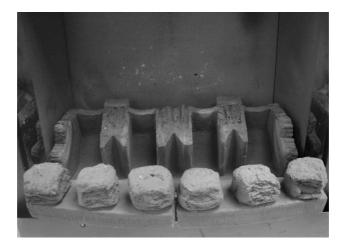
d) Fit four large coals behind the ceramic front rails as shown below in Fig. 5
